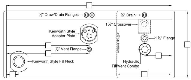
Please note: All sizes are NPTF unless otherwise noted and reference all measurements from the lateral weld seam and the end cap weld seam to the center of the fittings.
